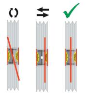
It is important that the pulleys are mounted correctly on the shafts and that the shafts are straight before starting the alignment process. Wobbling or warped pulleys affect the alignment quality severly.
