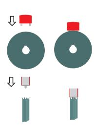
Position both units with the spring action probes resting in the same grove on both pulleys and the units are facing each other as shown below.
